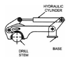
With this breakout wrench, the operator can comfortably and safely sit in his cabin and easily break the stubborn connections. The wrench automatically compensates for the drill stem wear within the size range.
